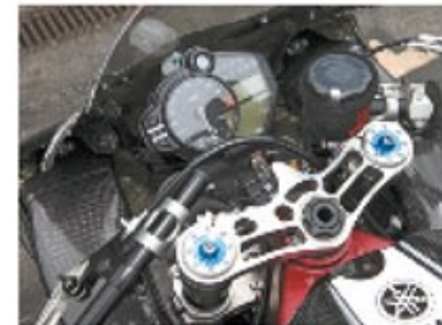
Gorgeous replacement yokes alter the steering geometry
